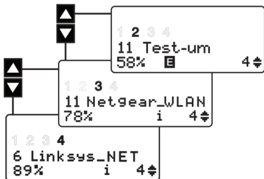
During scanning a ping is sent to the Internet IP every 15 seconds. If a response is received, an Internet indicator (i) is displayed.
