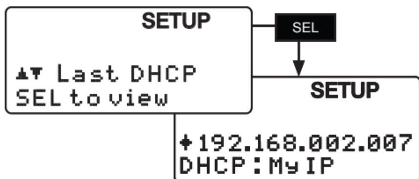
Use the up and down arrow keys to scroll through the Last DHCP items. Press SEL to view an item's MAC address. Since most wireless networking hardware has a visible MAC address label, this allows the components of the wireless network to be identified more easily.
