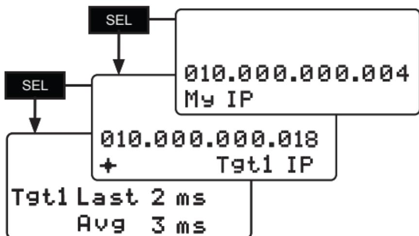
The Ping Target IPs can be viewed and edited from this display. The Internet IP can only be edited from the Target Setup submenu during Setup mode.
