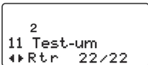
Use the left and right arrow keys to view the ping test results for the IP addresses associated with the WLAN selected, including the Router, DNS, target IP addresses 1-4, and the Internet.
