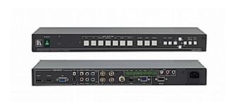
The VP-436N is a 7-input scaler/switcher for composite, component, s-Video (Y/C), computer graphics video and HDMI with unbalanced stereo and S/PDIF audio signals. It scales the selected video signal to a computer graphics or HDTV output resolution, embeds the audio and outputs an HDMI signal.
