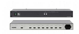
The VM-8HDMI is a distribution amplifier for HDMI signals. It reclocks and equalizes the signal and distributes it to eight identical outputs.
