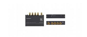
The VM-4HD is a high performance distribution amplifier for SDI (SMPTE 259M and SMPTE 344M) and HD-SDI (SMPTE 292M) signals. It takes one input, provides reclocking and equalization and distributes the signal to four identical outputs.
