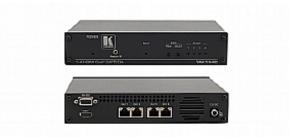
The VM-1H4C is a high-quality twisted pair distribution amplifier for HDMI signals. The unit receives serial commands and IR signals transparently via the RS-232 port and the TP link. It reclocks and equalizes the input signal and distributes it to four DGKat TP outputs.
