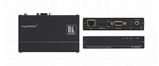
The TP-580T is a high-performance, HDBaseT twisted pair transmitter for HDMI, bidirectional RS-232 and IR signals. The TP-580T inputs HDMI, RS-232, and IR signals and converts them into an HDBaseT twisted pair signal that it transmits to a TP-580R receiver.
