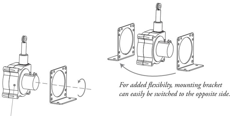
To change measuring cable direction simply remove the 3 bracket attaching screws and rotate sensor body to desired direction.
