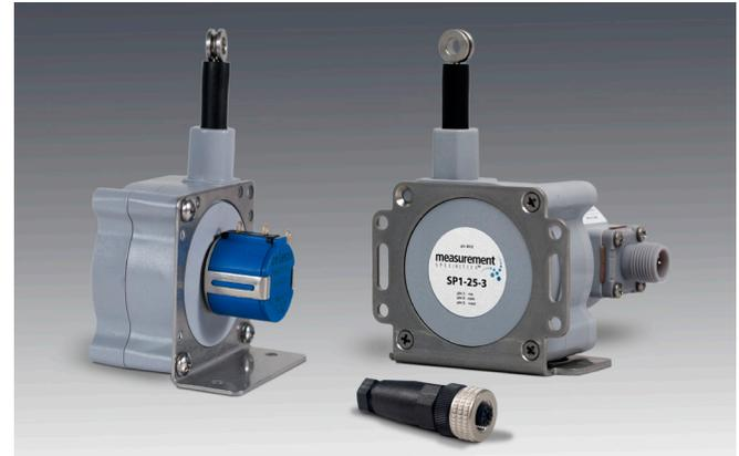
This compact stringpot with “voltage divider” output, provides ease-of-use and flexibility for measurement ranges up to 50 inches. Made of rugged polycarbonate, the SP1 fits in small spaces, doesn’t need perfect alignment and ships with a stainless steel mounting bracket to let the user easily orient this sensor in just about any direction imaginable.
