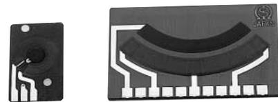
(Direct coating of conductive plastic paste was made on the flexible sheet.)
