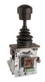
Example S22L S5 т - 3 Z P - A050 P134 - X **Basic unit** S22L left **Control-handle extended** -20 mm Grip / palm grip Dead man Axis 1 (direction 1-2) 3 3 contacts (2A 250 V AC15) Ζ Spring return Potentiometer Description axis 1 (direction 1-2) Arrangement MSP21-0 A050 P134 Potentiometer T396 2 x 5 kOhm Special model Special / customer specified
