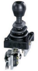
Example S1 - A05 P374 Т - 2 Z P - X **Basic unit** 1-axis Grip / palm grip Dead man Axis 1 (direction 1-2) 2 contacts (1,5A 24 V DC13) Z Spring return Potentiometer Description axis 1 (direction 1-2) Arrangement MSP21 P374 Potentiometer T 375 2 x 5 kOhm Special model Special / customer specified
