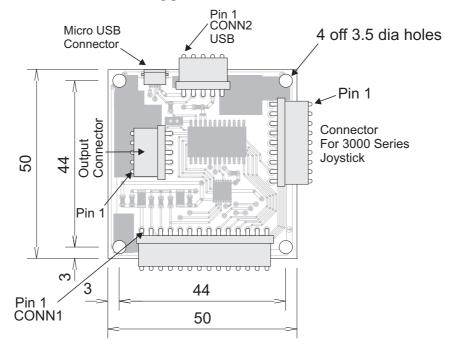
USB connection is made via either a 5 way 2.54mm pitch Molex® KK style header or a Micro USB type B socket on the board. A suitable USB cable (1.5m long) is included.
