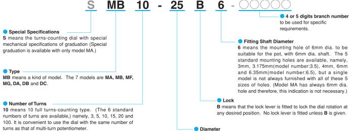
**25** means the approximate outer diameter of the dial body in metric system. (The 8 standard diameters are available,) namely, 15mm, 22mm, 24mm, 25mm, 26mm, 27mm, 46mm and 55mm.
