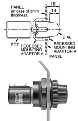
Note: 1 pc. each of mounting nut and rubber washer are attached.
