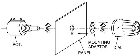
The mounting adaptor of Model DA Series Digital Counting Dial and the Helicalohm pot. are fixed on the panel according to the illustration given left. The shaft of the Helicalohm pot. is turned anticlockwise to its limit and is put into the mounting hole of the dial which was already set at "000". The shaft of the Helicalohm pot. is secured by the screw positioned at the knob of the dial with the attached hexagonal wrench. With this, the mounting is completed.
