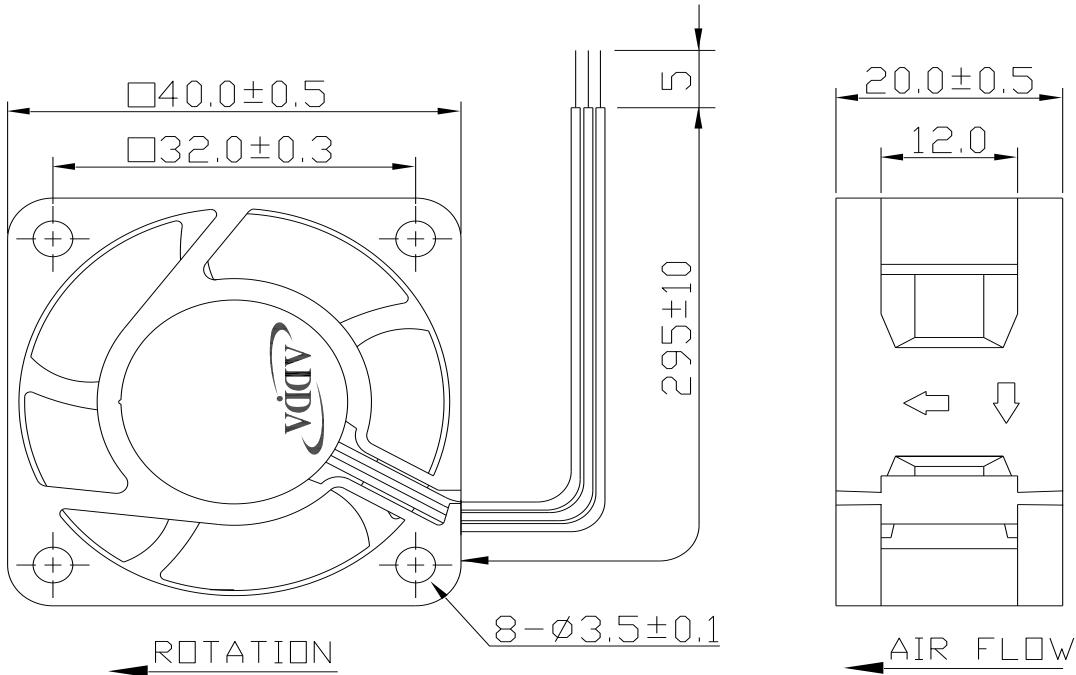
LEAD WIRES : UL 1007, AWG26, L = 295 +/- 10 mm
