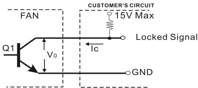
\*Transistor Q1 at "ON" position
