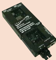
Piggy-Back Power Supply Attached to Converter
