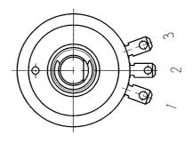
The output ratio from the wiper contact is 50% when the flatted area on the shaft is positioned as illustrated
