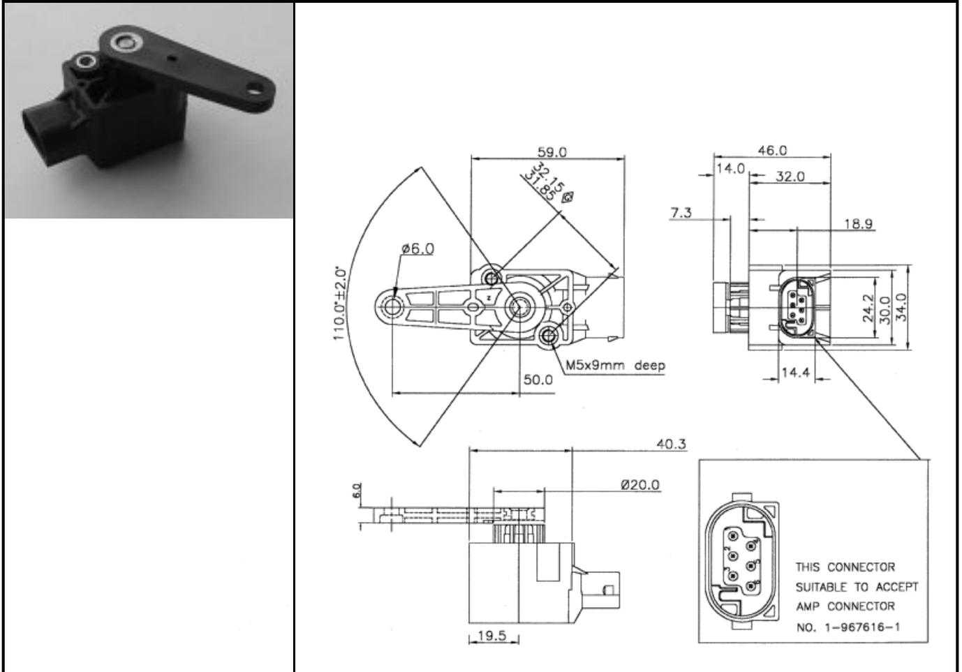
A Multi-function sensor based on the Industry Standard package size for use in Suspension Control and Headlamp levelling. The sensor has the option of single or dual potentiometer track outputs and has a capability of having an integral electronic signal conditioning unit.
