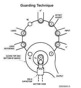
Use 10-pin layout. Guard around C<sub>h</sub>is tied to output.
