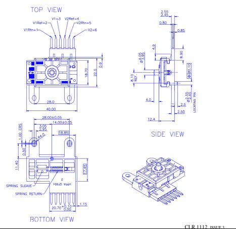
Integrated Position Sensor with option of single or twin potentiometer track outputs. Suitable for integration into customer mouldings to facilitate a sealed construction. The Sensor can be used in Small Engine Management Systems, Throttle Position Sensing, Seat Position, Pedal Position and is suitable to replace discrete Track & Wiper systems
