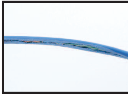
2. Commercial cable after 25 cycles.
