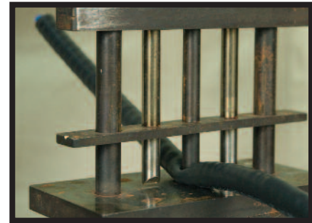
A chisel-point mandrel on an Instron machine performs the cut-through procedure.
