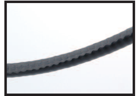
3. Industrial cable after 25 cycles.
