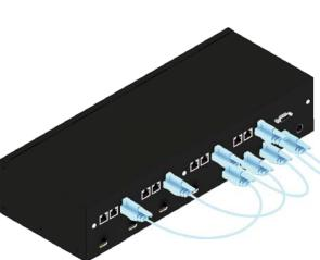
When all jumpers are connected, extension for each HDMI output is possible. If a local display is going to be used, simply do not use that HDMI output port's jumper and extension connection.
