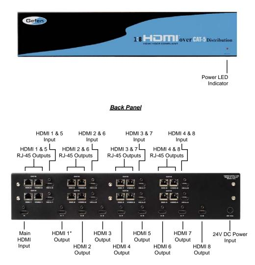
\*NOTE: Display information (EDID) is used from whichever display is connected to this port.
