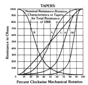
Tapers A, DB, S and U are measured between the wiper and the counter-clockwise terminals: taper B is measured between the wiper and the clockwise terminals.
