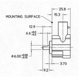
1 Connector mates with Packard Electric METRI-Pack 150 series, pull-to-seat 6 pin sealed connector assemblies.
