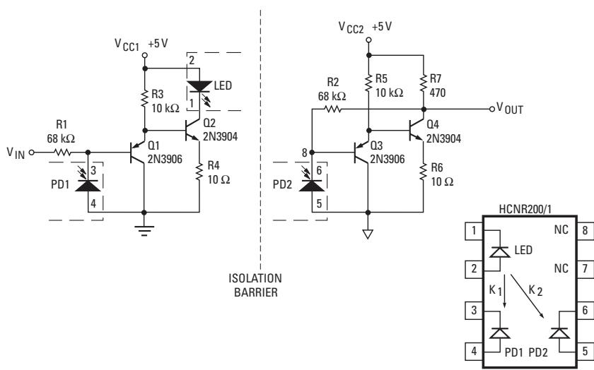
This is a high-speed, low-cost isolation amplifier for use in the feedback path of switch-mode power supplies or motor speed and position measurement. This circuit can be used in applications where high bandwidth, low-cost, and stable gain are required.
