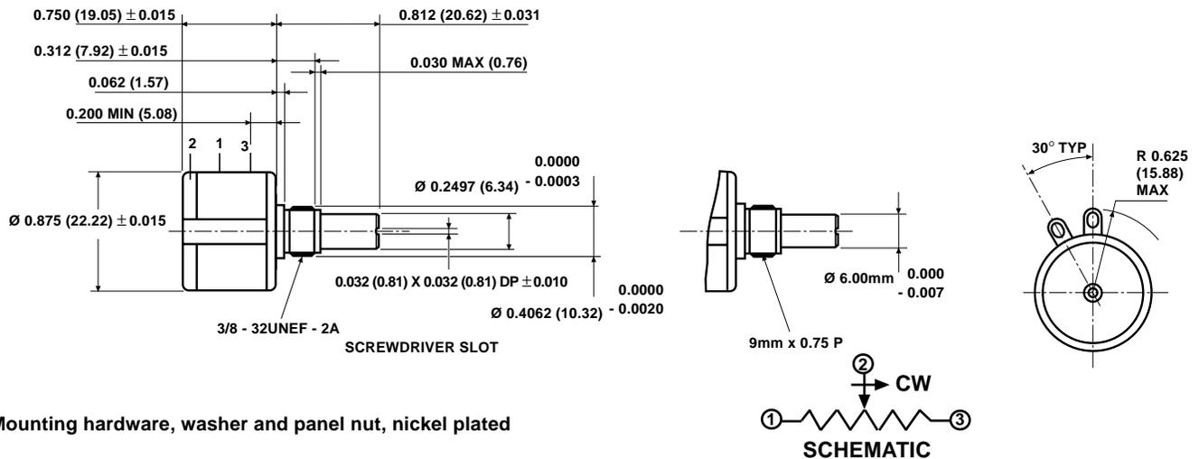
Mounting hardware, washer and panel nut, nickel plated
