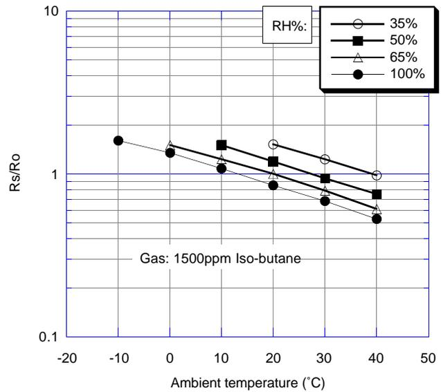
Fig. 6 - Temperature and humidity dependency ( $R_s/R_o$ )
