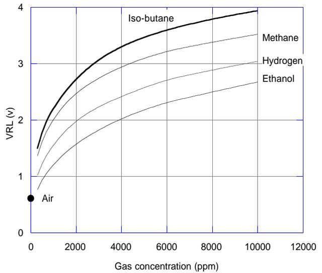
Fig. 5 - Sensitivity to various gases (VRL)
