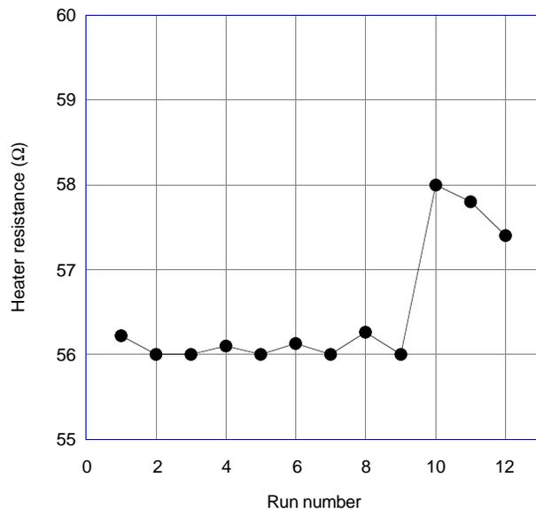
Fig. 17 - Effect of gas exposure on heater resistance
