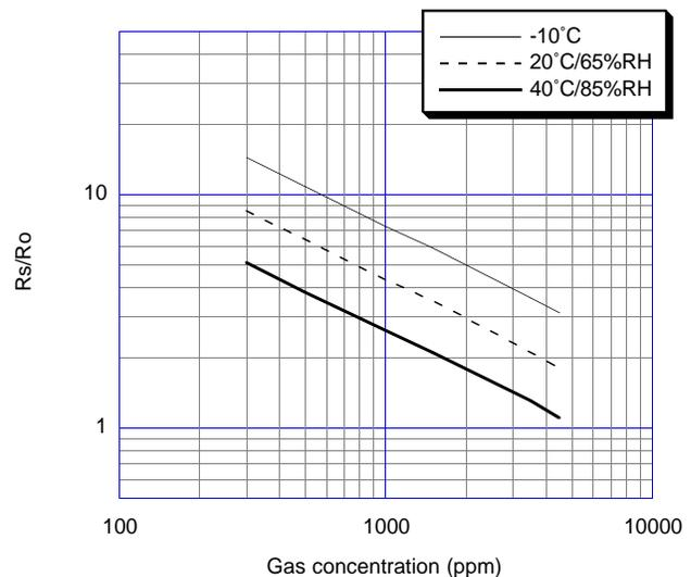
Fig. 7 - Resistance change ratio under various ambient conditions
