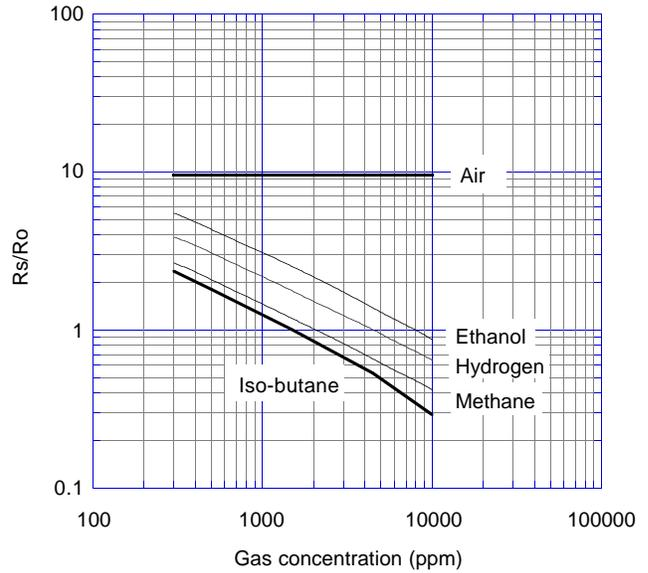
Fig. 4 - Sensitivity to various gases ( $R_s/R_o$ )
