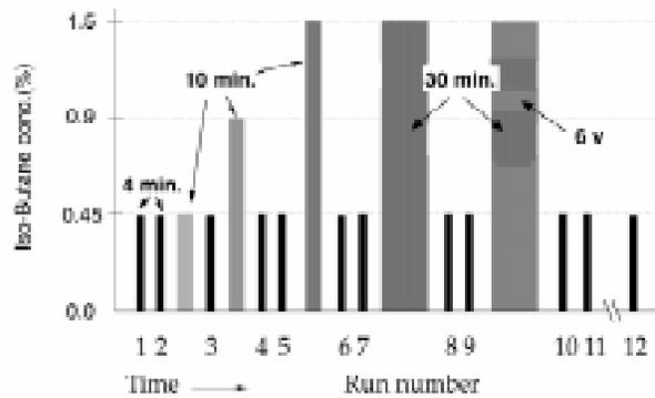
Fig. 15 - Test procedure for gas exposure
