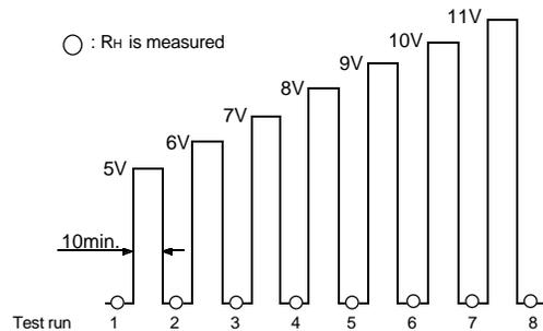
Fig. 21 - Test procedure for heater durability
