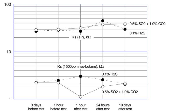
Fig. 19 - Corrosion test
