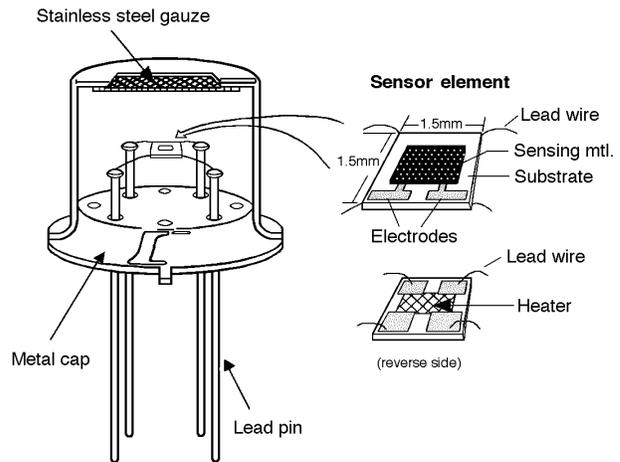
Fig. 1 - Sensor structure
