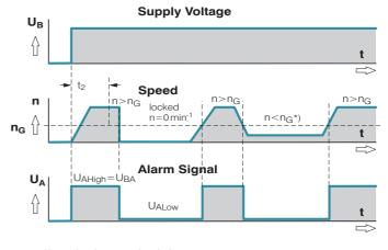
$t_2$  = Alarm signal suppression during start-up \* n < speed limit n<sub>G</sub> by braking or blocking.
