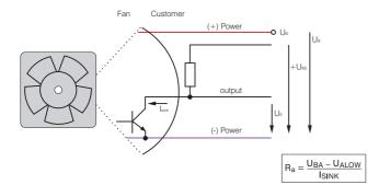
All voltages measured to ground External load resistance  $R_{\text{a}}$  from  $U_{\text{A}}$  to  $U_{\text{BA}}$  required.
