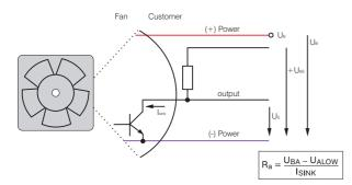
All voltages measured to ground External load resistance Ra from  $U_{\text{A}}$  to  $U_{\text{BA}}$  required.
