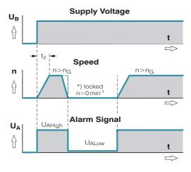
$t_2$  = Alarm signal suppression during start-up \* n < Speed limit n<sub>G</sub> by braking or blocking.
