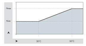
$\begin{array}{l} n_{\text{min}} \approx \ ^{1} /_{2} \ n_{\text{max}} \\ T_{\text{min}} \approx \ 30 \ ^{\circ}\text{C}; \ T_{\text{max}} = 50 \ ^{\circ}\text{C} \end{array}$
