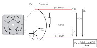
All voltages measured to ground. External load resistance  $R_a$  /  $U_S$  /  $U_{BS}$  required.
