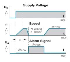
$t_2 = A larm \mbox{ signal suppression during start-up} \\ ^* \mbox{ n } < \mbox{ Speed limit } n_6 \mbox{ by braking or blocking}$
