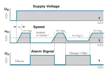
$t_2 = \text{Alarm signal suppression during start-up} \\$
