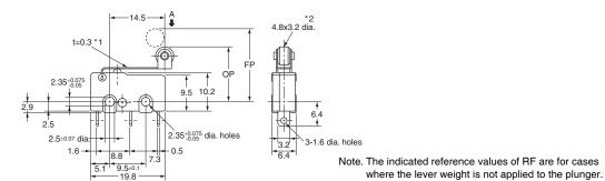
\*1. Stainless-steel lever \*2. Polyacetal resin roller
