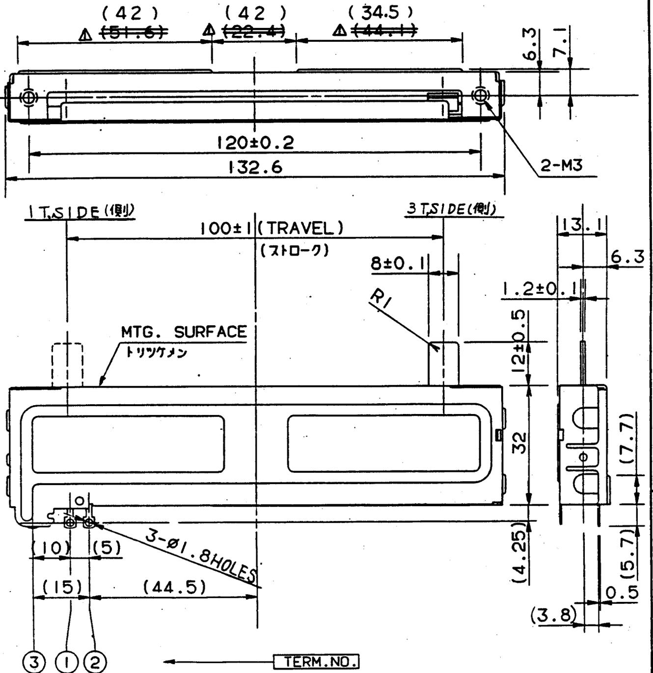
NOTE 1. MOUNTING SCREW THREAD LENGTH IS CHASSIS THICKNESS+4MM MAX.
