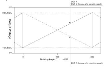
Special Specifications Available. (In case of the potentiometer with special specifications, the general specifications and environmental specifications may change. Please consult us in advance.) Special effective electrical angle(90°,180°,270°- arbitrary angles), Special machining on the shaft, Special output (Cross, parallel, Dual independent output), Special applied voltage(12V,24V), PWM output, Low current consumption in slow mode.
