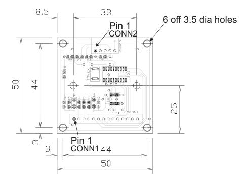
USB connection is made via a 5 way Molex KK style header on the board. A Suitable USB cable (1.5m long) is also available - Part number 919998. The joystick connects to Conn1, a 14 way molex KK style header. Please refer to the pin-outs below:
