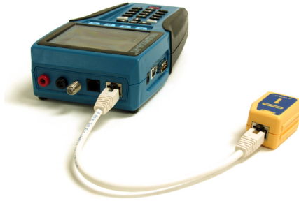
Figure 7. Wiremapper Remote #1 Connected to Validator-NT
