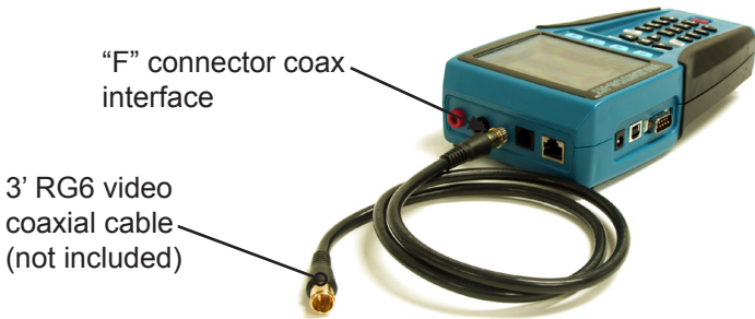
Figure 4. Video Coaxial Cable Connected to Validator-NT
