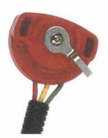
Conductive polymer potentiometer for automotive and other similar demanding applications. A high performance cost effective potentiometer, with long endurance life and protection from engine compartment environment. Termination via 280 mm long flying leads.
