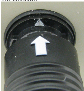
Arrows on power supply connectors
