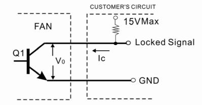
\*Transistor Q1 at "ON" position Collector current........ $I_c$ =5mA Max Saturation Voltage...... $V_{oL}$ =1.0V Max (Between Collector and Emitter at  $I_c$ =5mA) \*Transistor Q1 at "OFF" position Release Voltage...... $V_{OH}$ =15V Max
