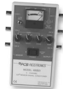
Model 480B21 3 channel, triaxial, gain x1, x10, x100
