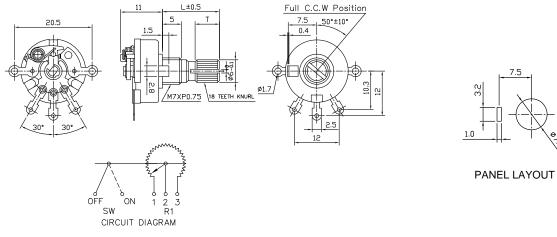
MODEL P170N2 (Side Adjust, PCB Pins)
