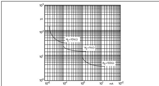
FIGURE 2. Rise and fall times of phototransistor.
