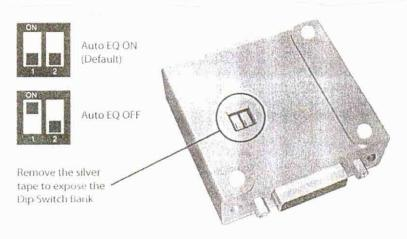
By default, both Dip Switches should be in the off position as shown above. To disable the Auto EQ, please flip Dip Switch 1 to the ON position. You must then proceed to manually adjust the EQ by turning the EQ trim pot on the front of the unit is small increments. It is important to turn the dial in very small increments as the "sweet spot" at which all video noise is eliminated can be very small.
