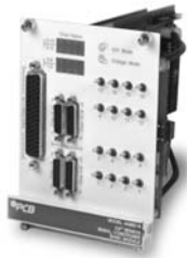
Model 442B216 16-channel, unity gain, with selectable ICP® or voltage mode
