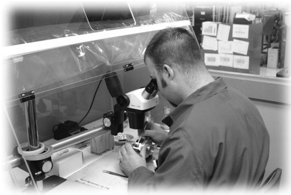
A “gaged” load cell structure is ready for final wiring of the sealed electrical connector.
