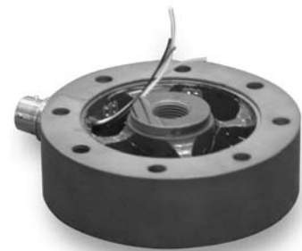
A “gaged” load cell structure is ready for final wiring of the sealed electrical connector.
