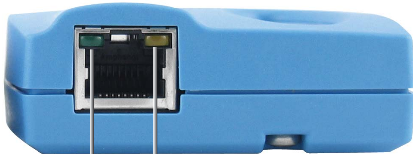
Device LED (green) Link LED (yellow)
