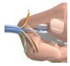
Lay each twisted pair into the tool channel with the pair ends facing toward the pick. Place your thumb on the thumb notch to stabilize and secure the pair. The tip of the pick should rest in the webbing between the two conductors. While holding the pair in place with your thumb, puncture the pair webbing with the pick.
