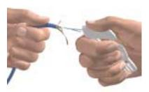
Holding the cable in one hand, with the hand holding the tool, pull the tool away from you, allowing the pick to separate the conductors of the pair.
