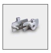
Z 103 g 2.5 Z 103 g 3 Fork coupling with low backlash for shaft diameters 2.5 mm or 3 mm. Stainless steel, ground driving pin. Mounting with 1 fillister head screw M 2 each with
